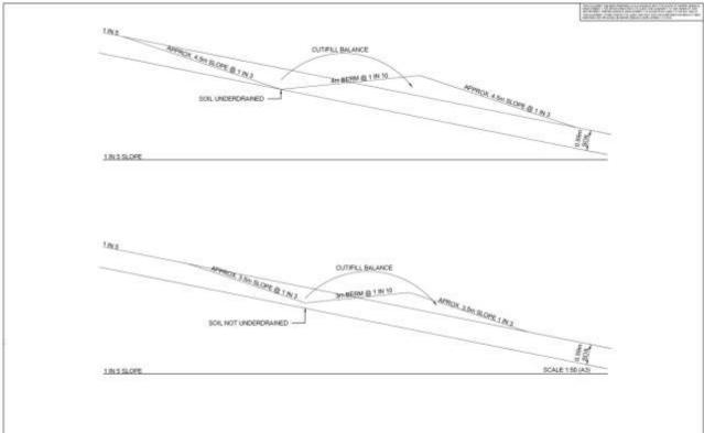
Example cross-sectional views of the contour berms, which will form the water management systems, as well as potential options for future access to assist in deer management, maintenance and public access.
