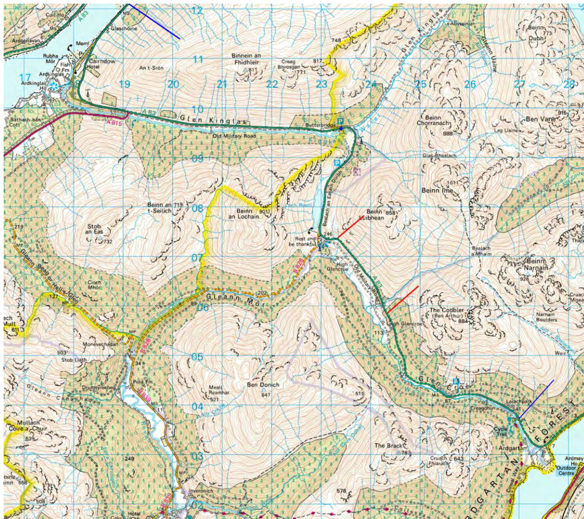
Figure 1. Map showing the notional geographical limits of debris flow occurrence affecting the A83 trunk road in the general area (blue lines) of the Rest and be Thankful and the approximate limit for events since 2007 (red lines). Reproduced by permission of Ordnance Survey, on behalf of HMSO, © Crown copyright and database rights, 2012. All rights reserved. Ordnance Survey Licence number 100046668.
